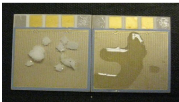
Fig. 1 DEA electrodes with anthracene in crystalline form ( left ), and amorphous form ( right )
